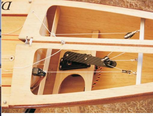
PORT inside of for ship Single brock Bulk head w. snackle (614) (Cockpit) Eye bolt PTFE Jain lead (52a) for decktrack (38a) Jeb sheet € 40 mm Arm -Servo CENTER (K-Bits) LINE < Deck track from SAILSEC Main sheet (286) Tube for leading sheet through bulk head of set to align sheets (skacklers removed) (616) with tubes Scale 1:1 New hole for blocks, 15mm in from original hole STAR BOARD
